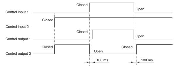
Control input 2 is disabled while the control input 1 is being closed. The control output 2 becomes closed when the control input 1 is opened.
