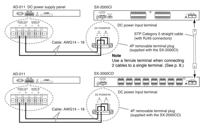
**Note:** When using the AD-031B DC power supply panel (optional), make connections in the same manner.
