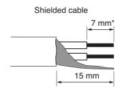
\* Expose 8 mm or more when using the above ferrule terminal, and cut off an extra conductor protruding from the sleeve.
